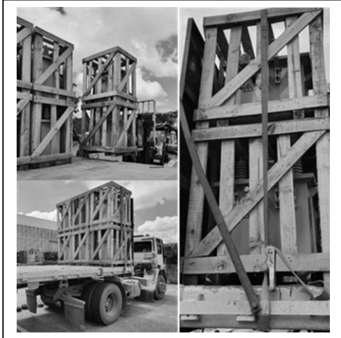
Figure 17: Loading and securing the first row
