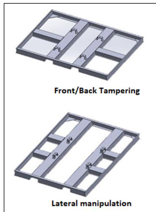
Figure 13: Metal base for power transformers
