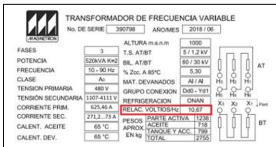
Figure 4-2: Example nameplate illustrating the V/Hz relationship
