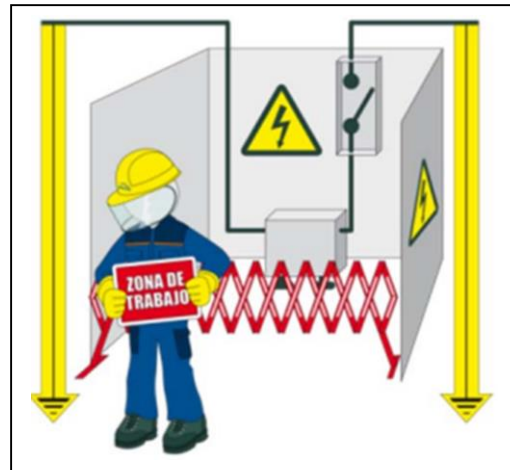
Figure 7: Short circuit and ground connection of HV and LV terminals
