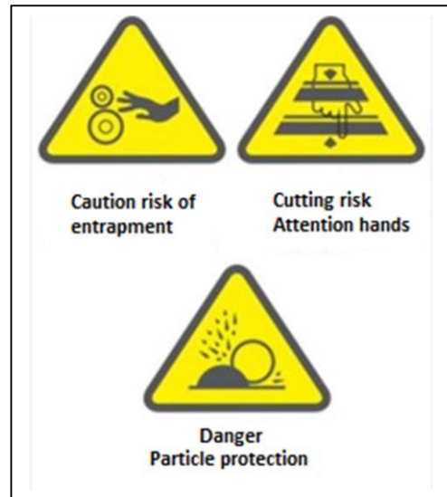
Figure 2: Signs of mechanical risk
