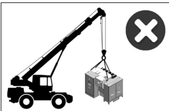
Figure 9: Prohibited from transporting the transformer from the lifting lugs
