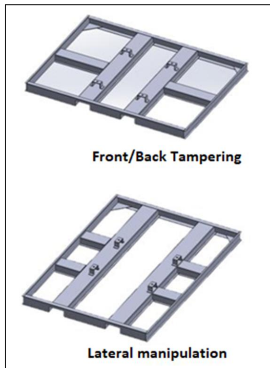
Figure 12: Metal base for power transformers
