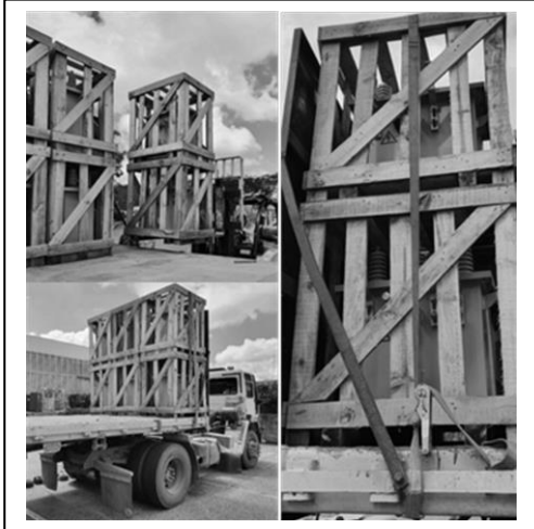
Figure 17: Loading and securing the first row
