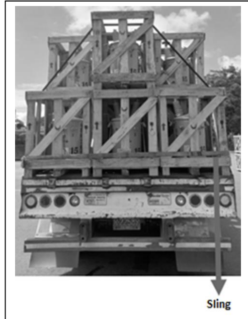
Figure 19: Securing the last row of loaded transformers
