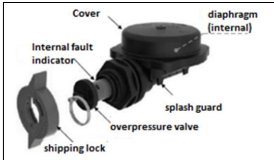
Figure 34: Parts of the IFD
