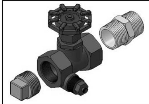
Figure 43: Drain/recirculation valve
