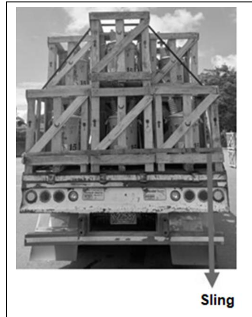
Figure 23: Securing the last row of loaded transformers
