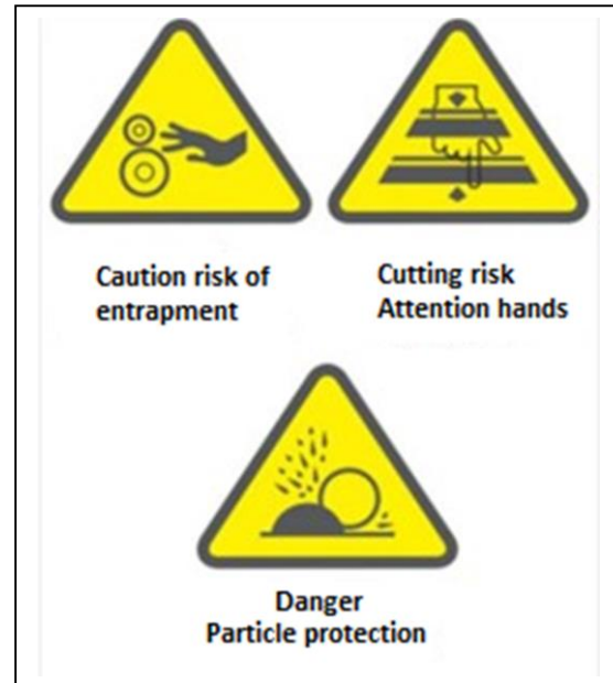
Figure 2: Signs of mechanical risk
