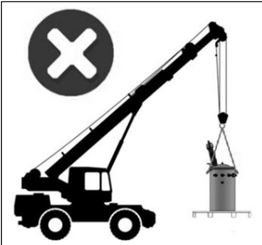
Figure 9: Prohibited from transporting the transformer from the lifting lugs
