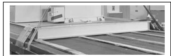
Figure 27: Boards between the base and the floor of the vehicle
