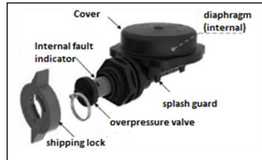
Figure 41: Parts of the IFD
