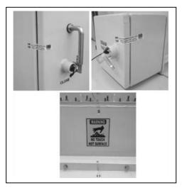
Figure 26-1: Security seal on removable parts
