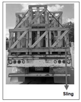
Figure 23: Securing the last row of loaded transformers
