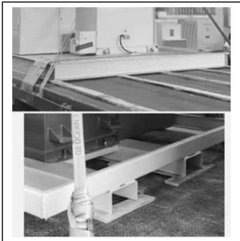
Figure 22: Wooden boards between the metal base of the transformer and the metal floor of the truck
