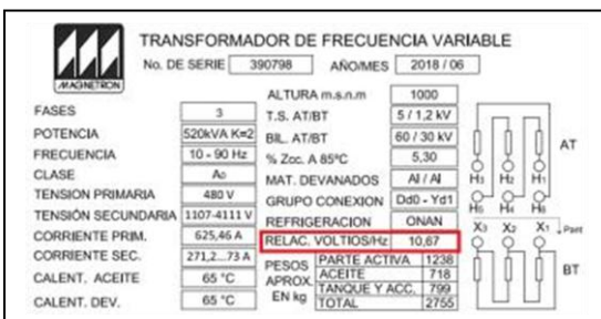
Figure 4-2: Example nameplate illustrating the V/Hz relationship
